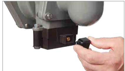
4. Remove the dust cover from the sensor.
